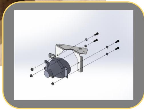
51. Re-Fit fog lamps to the Fog light brackets (B-0186L/R) using M6X16 Button head Bolts, Flat washers and Flange nuts from the Small Parts Kit.
