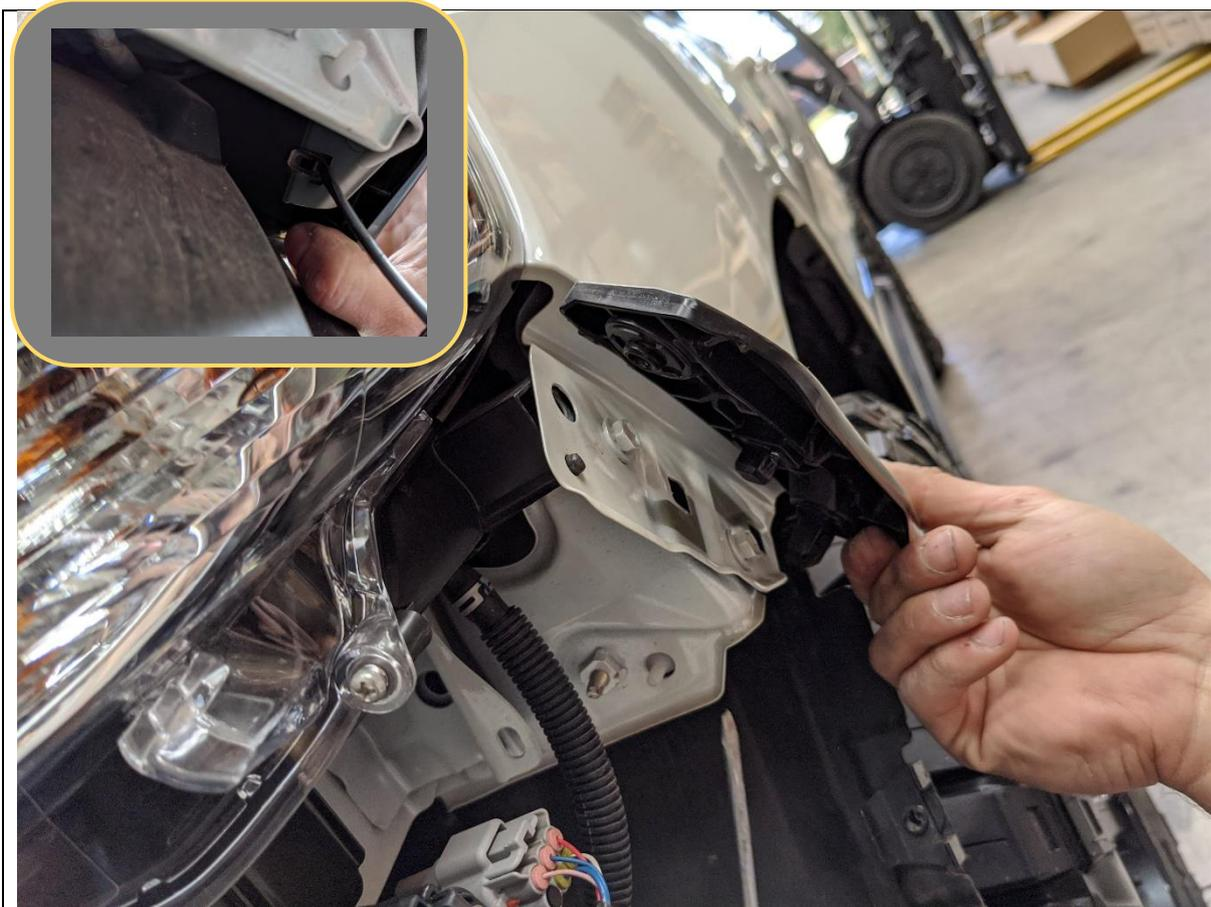
32. Remove the plastic bumper retainers by removing the Phillips head screw, then prying out the large clip from behind using trim tool
