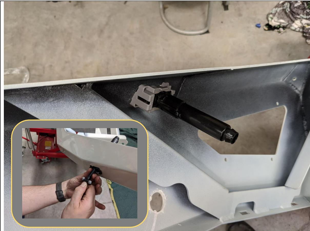
59. If Equipped Re fit headlight washers to bar.
