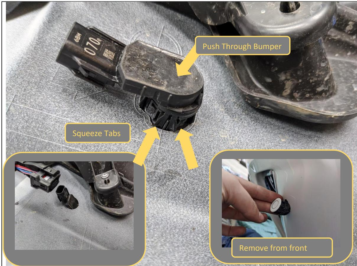
23. Disconnect the parking sensors from the loom by first prying open the plastic housing, then disconnecting the multi plug connector.
