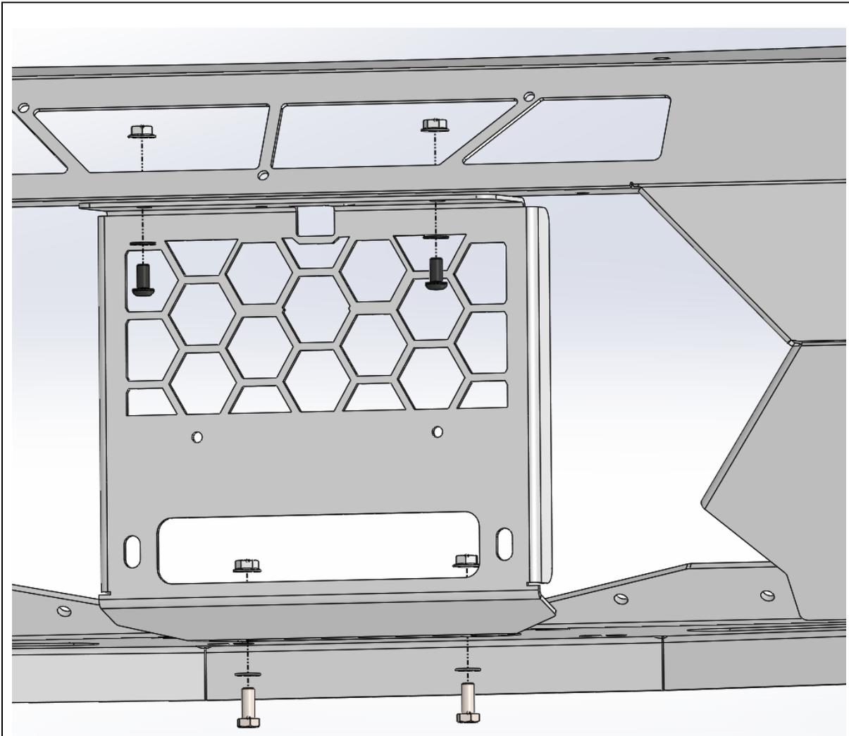
81. If Required, Fit winch fairlead to Mesh Fairlead Mount (M-0007). Use M10 or 3/8" Fasteners supplied with winch. The bar is only compatible with Hawse type fairleads.
