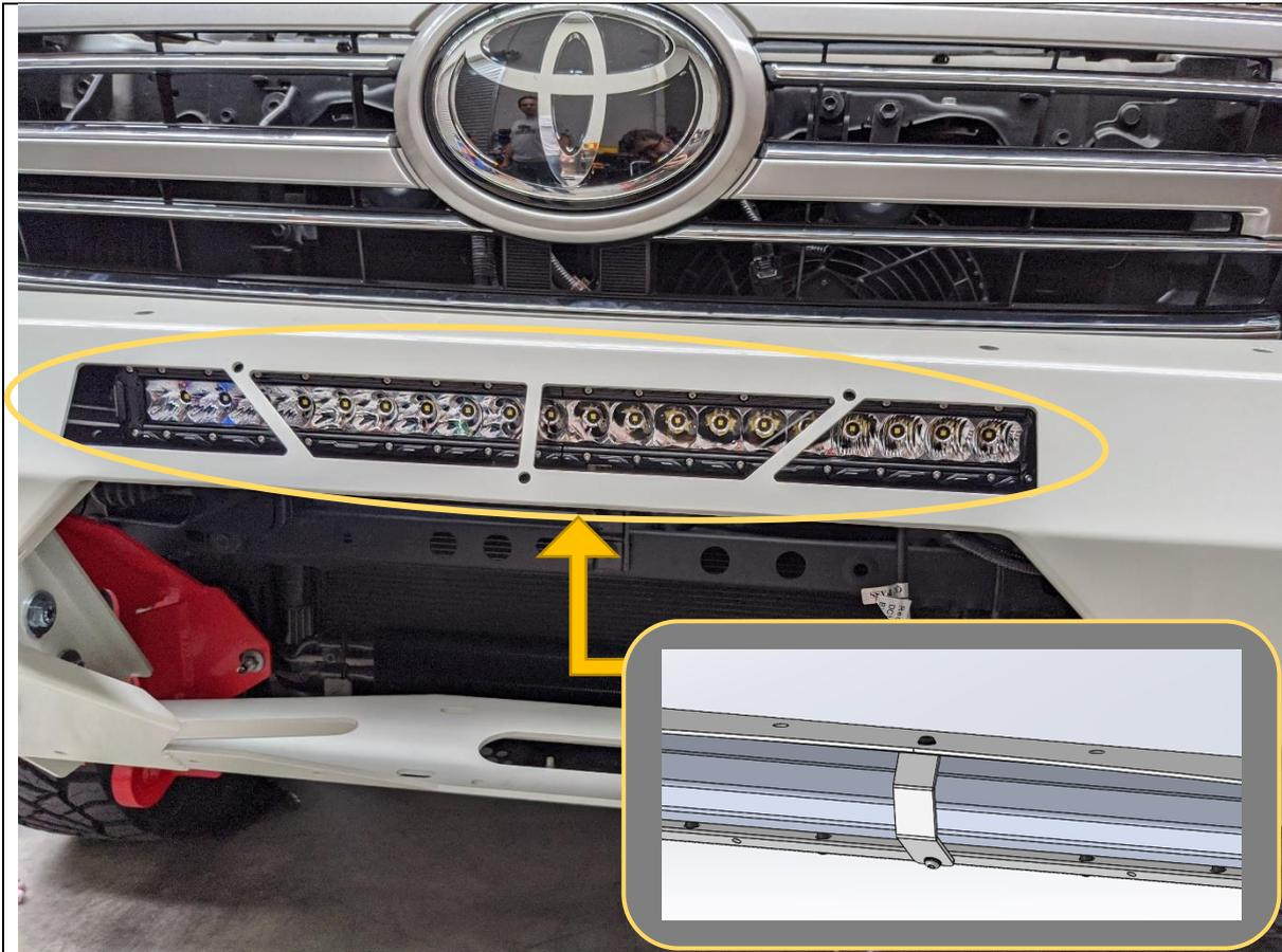
69. If Fitting an integrated light bar, do so now. Leave bolts loose at this stage to allow fitment of mesh panels.
