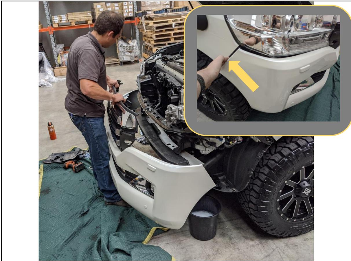
14. Starting from the wheel arch, carefully pull the bumper away from the body of the vehicle to release the clips.
