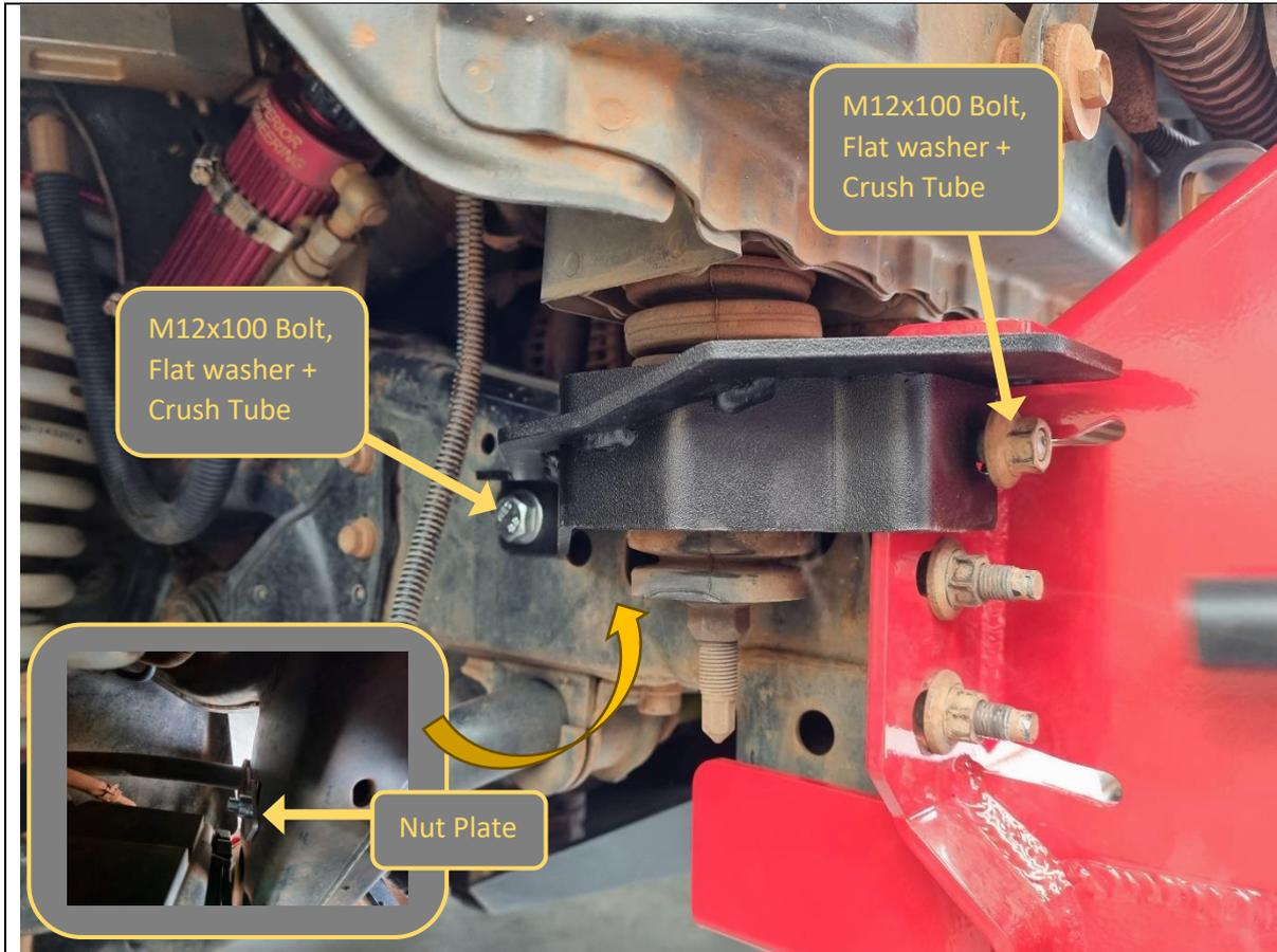
45. Fit the chassis brace between the impact assembly and the square slot in the chassis as shown, Secure at the front using the factory nut.
