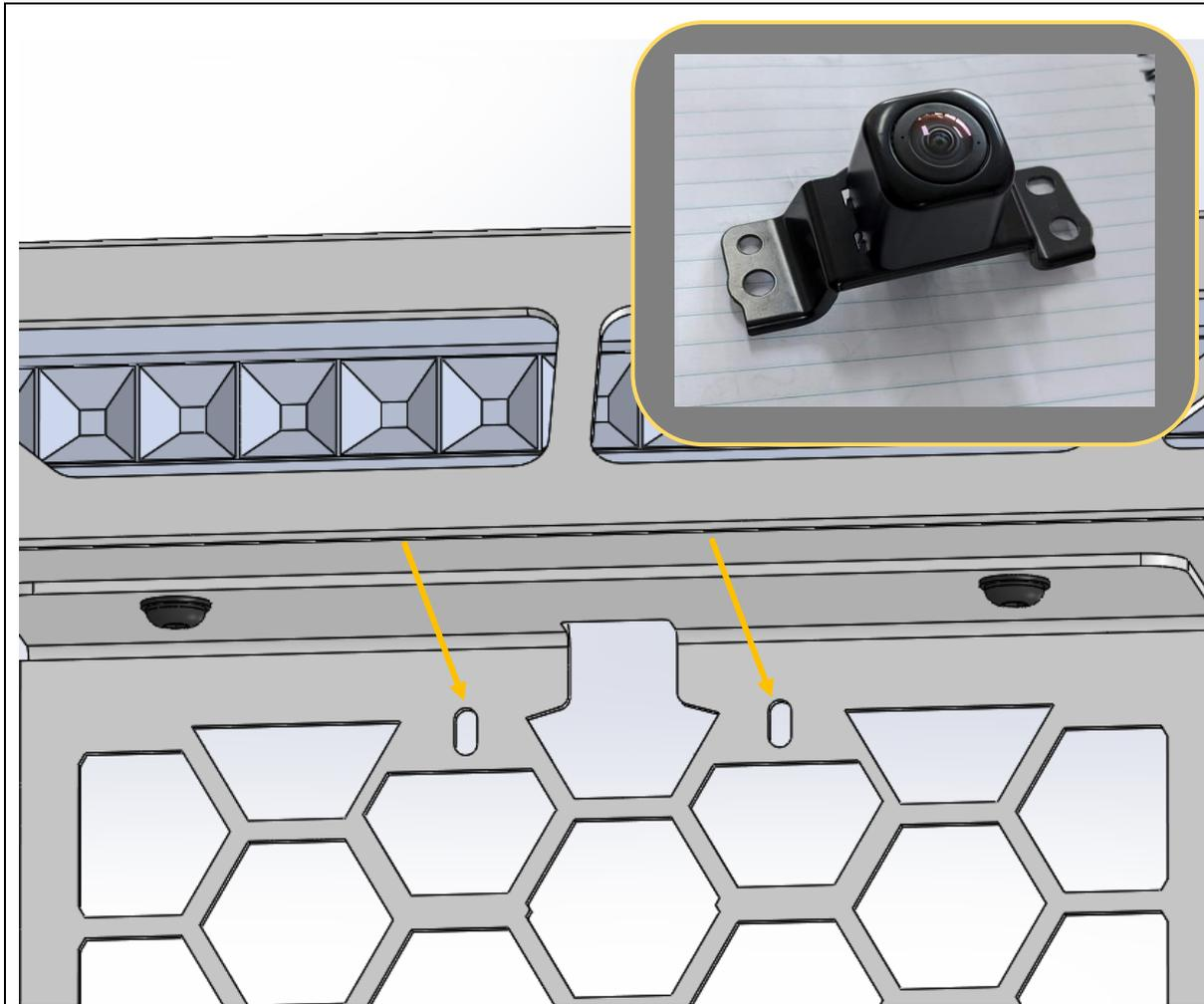
78. If vehicle is fitted with front camera, the bar will obscure bottom part of front camera image. Additionally, if a large light bar is fitted this will also obscure image in default badge location.
