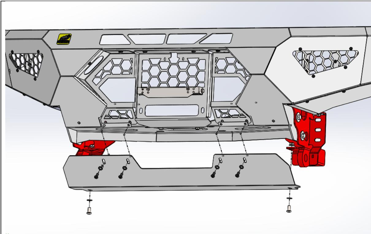
93. Fit Center Bash Plate (U-0011) using, M8x30 button head, flat washer and flange nut to front face. Ensure these fasteners pass through the side mesh panels also. Ensure the Shims are between the bash plate and mesh panels.
