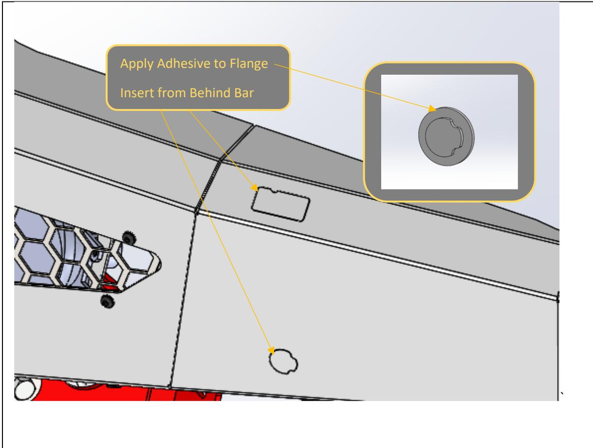
58. If not fitting sensors / washers install supplied plug plates, using Automotive grade adhesive
