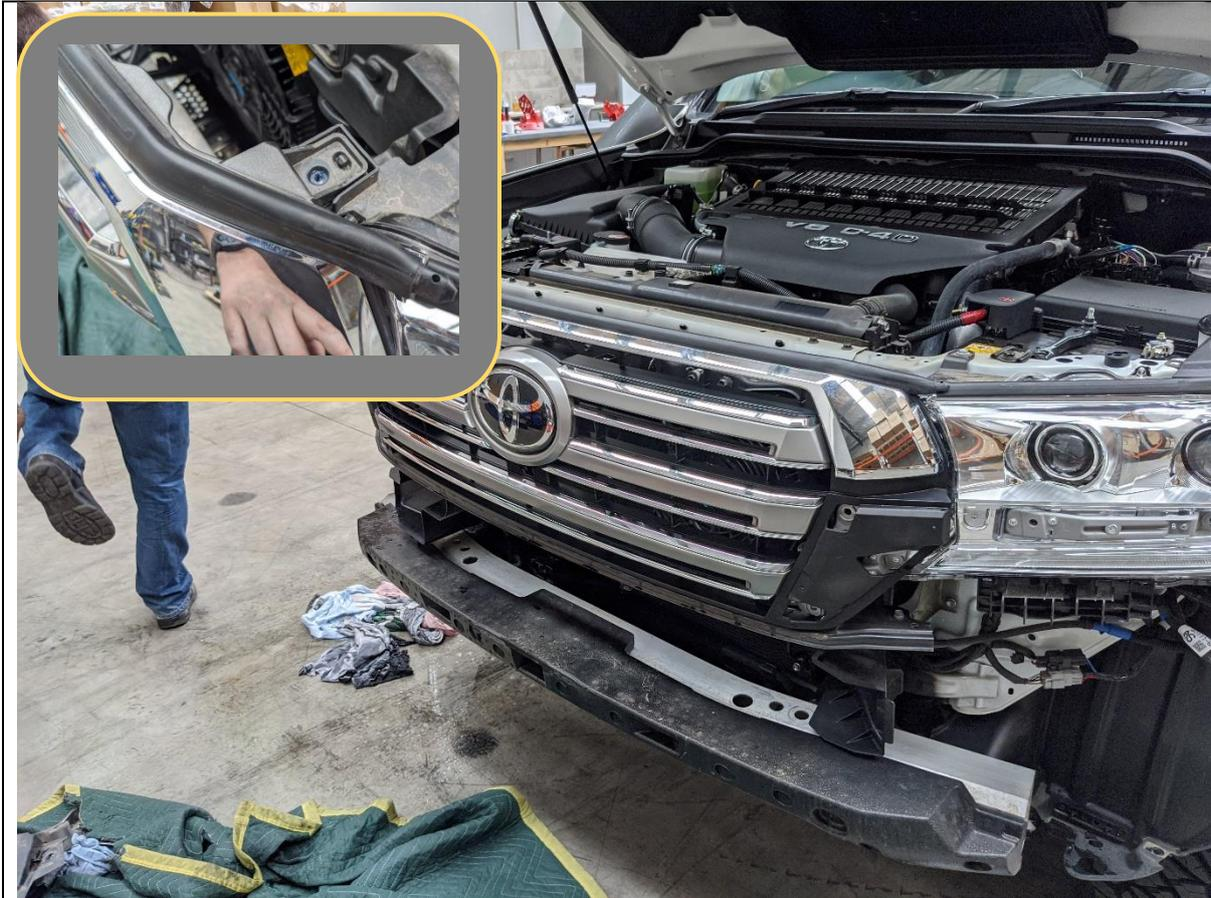
17. Re-Fit grille to vehicle, Secure the grille using the factory fasteners removed earlier.
