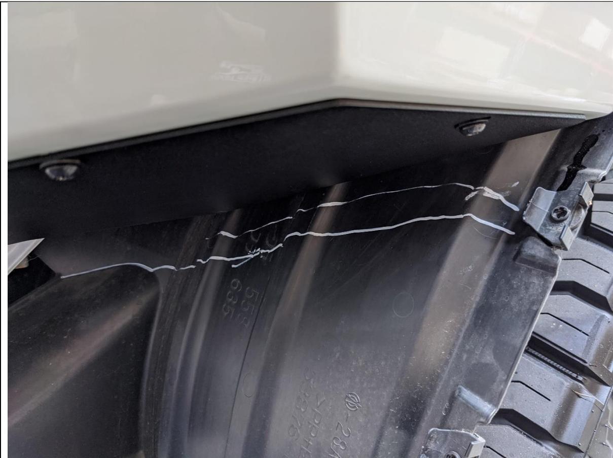
101. Using the edge of the under panel as a guide mark the wheel arch liner, approximately 15mm beyond the intersection of the under panel.
