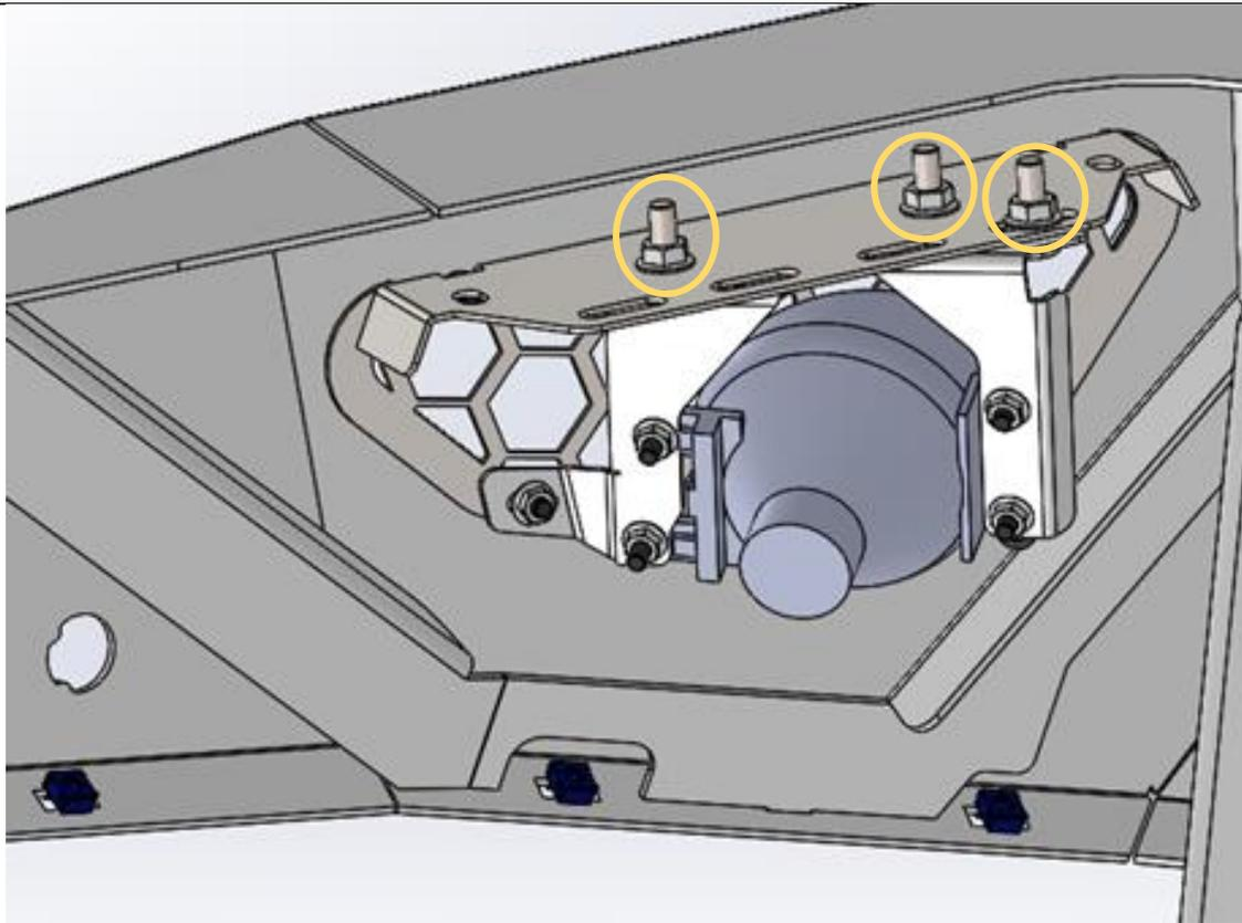
53. Fit fog light bracket, with fog light in place to the Mesh panel using 3x M8x25,
