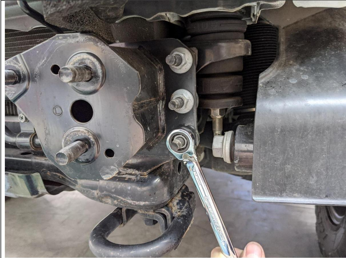
36. Remove Steel impact beam mounts by removing the 5x 14mm head flange nuts on each side.
