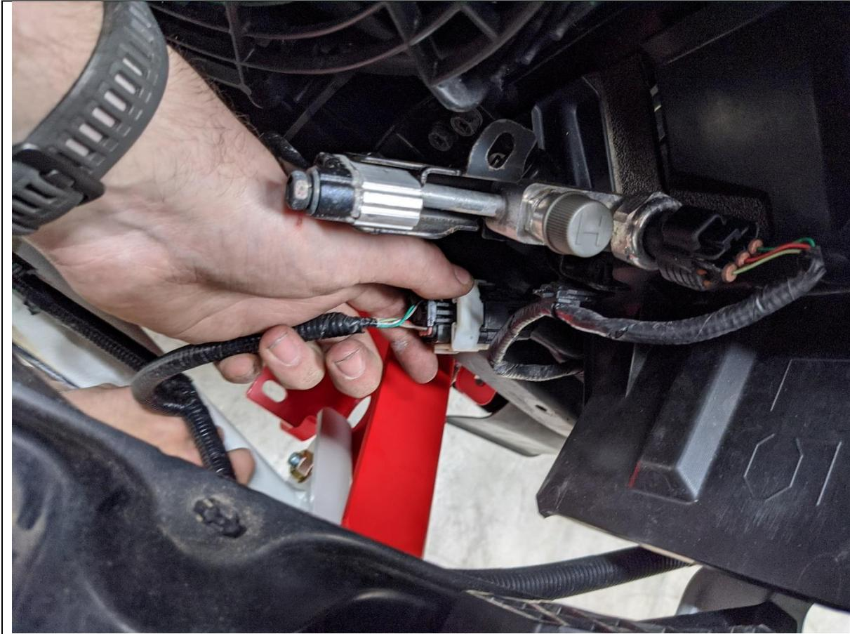
91. Re Connect Electrical Harness and headlight washers behind grille. If equipped also reconnect Radar and Camera harnesses.
