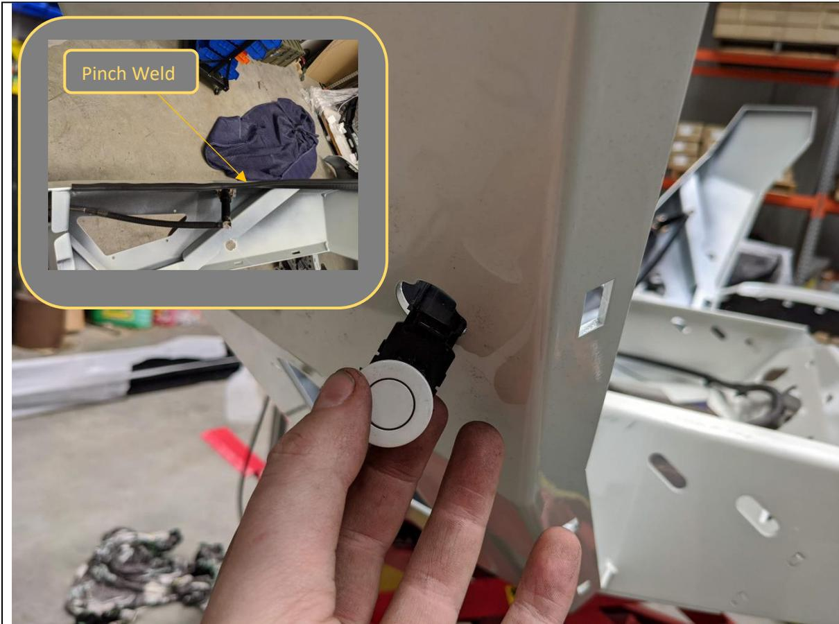
62. Re Fit parking sensors to the bar. Insert the sensor from the front of the bar. Push the sensor through and allow the tabs to expand and hold the sensor in place.
