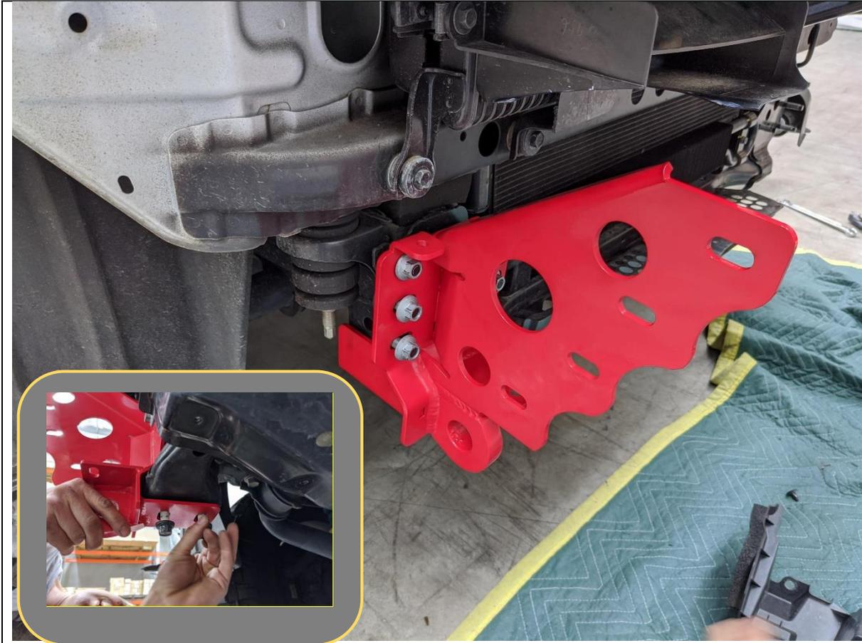
43. Fit the Impact mounts to the chassis, re using the original factory flange nuts (front) and Bolts (Bottom) as shown.
