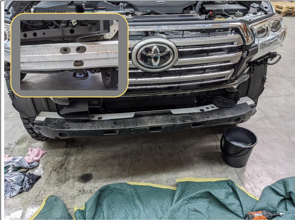
29. Remove the foam covering the impact beam assembly by lifting it off.
