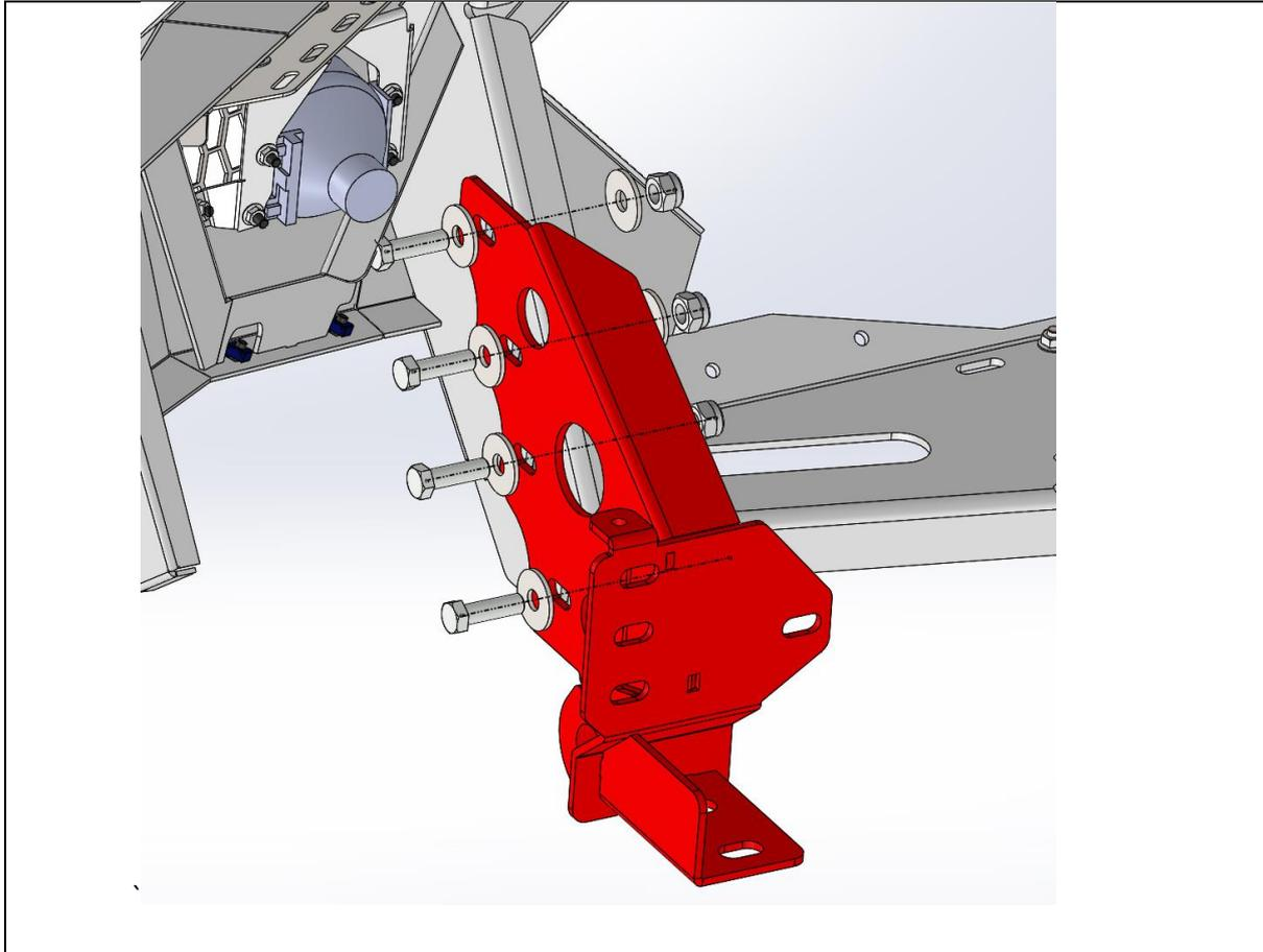
65. With assistance, either from another person, or a lifting trolley, lift the bar onto the mounts on the vehicle.
