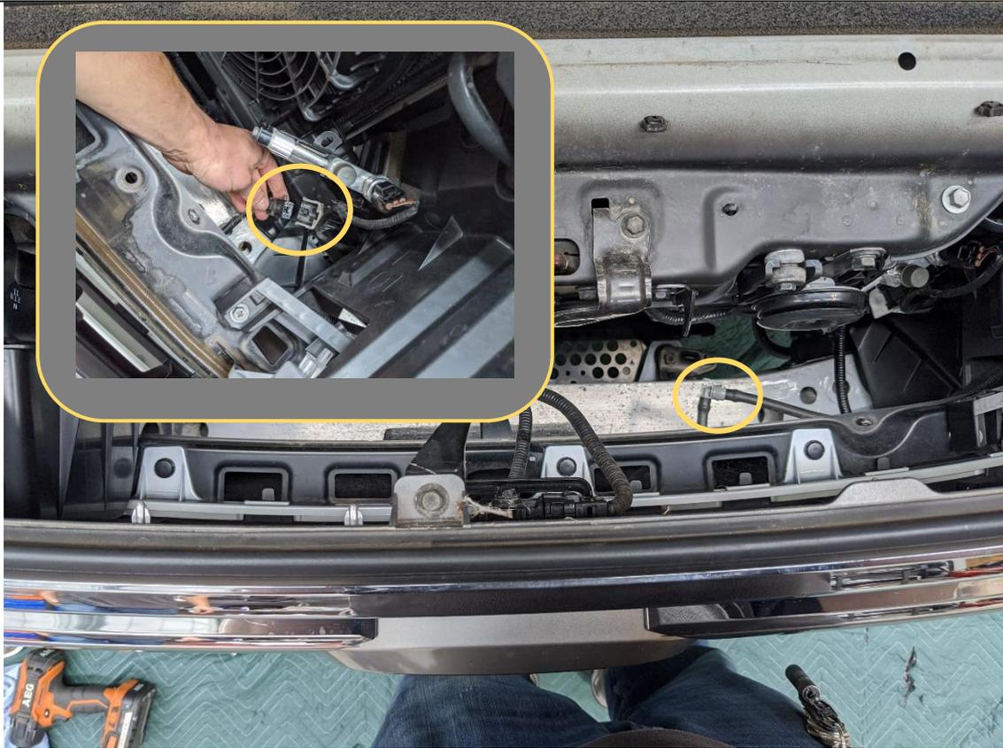
11. Disconnect the main electrical harness, located on the LHS of vehicle near bottom of grille.
