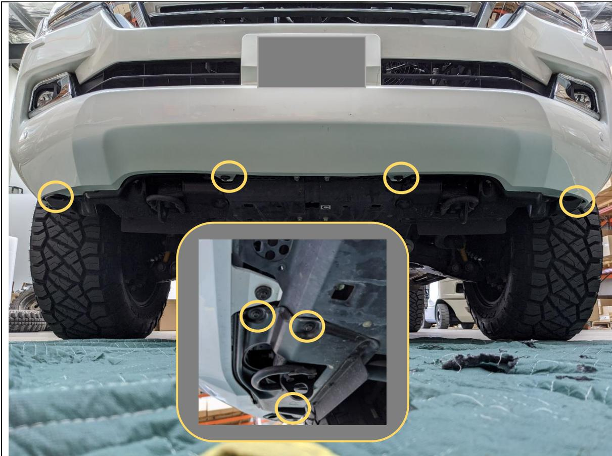
7. Remove the 10mm head screws securing the bumper to the underbody bash plate.
