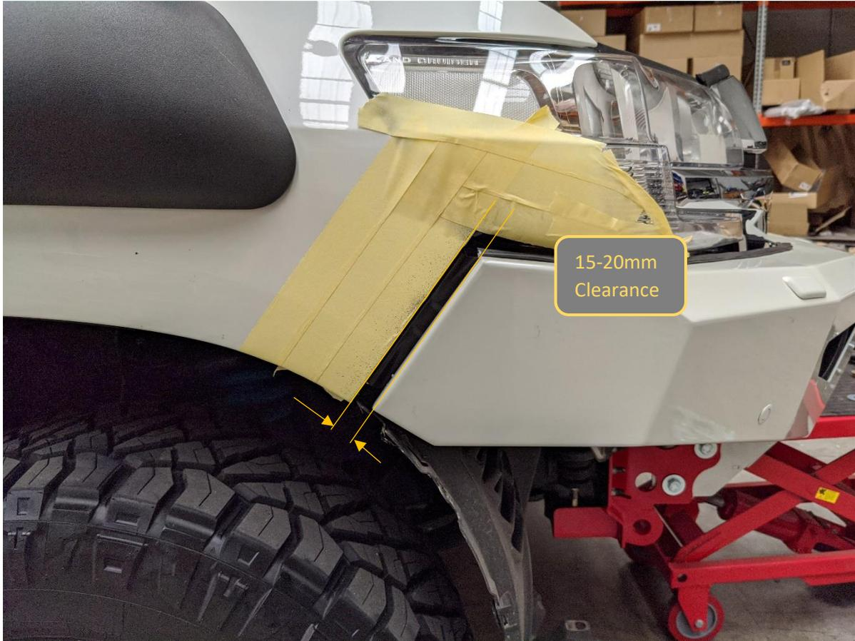
67. With assistance, from another person, Align the bar with the edges of the vehicle. Adjust such that the clearances are neat and even side to side.
