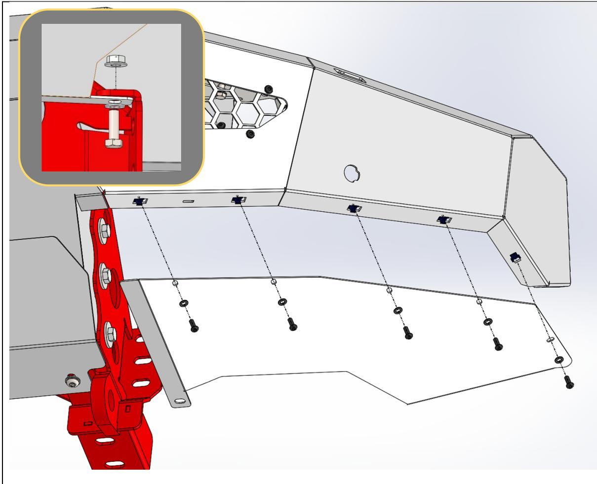
97. Fit Side Underpanels (U-0008L/R) using, M6x16 button head and flat washer into the cage nuts placed earlier.
