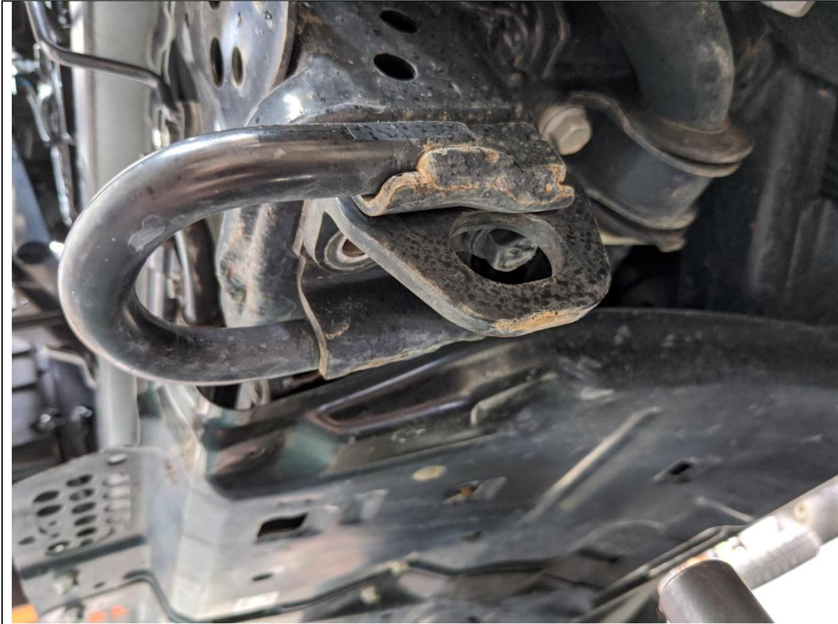
38. Remove the Factory tow point, by removing the 17mm head factory bolts.
