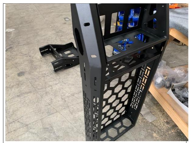
5. Slide side arm assembly over centre basket as shown and loosely fit M8 hardware to keep arm attached. Leave all hardware loose
