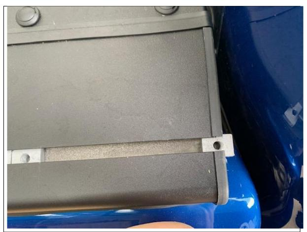
20. Fit small rectangular nuts into slot on roller shutter (6) per side
