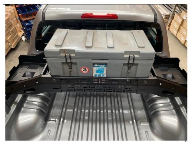
32. IF fitting centre space case, secure down with ratchet strap running from handle to handle underneath rack so you can still open the box
