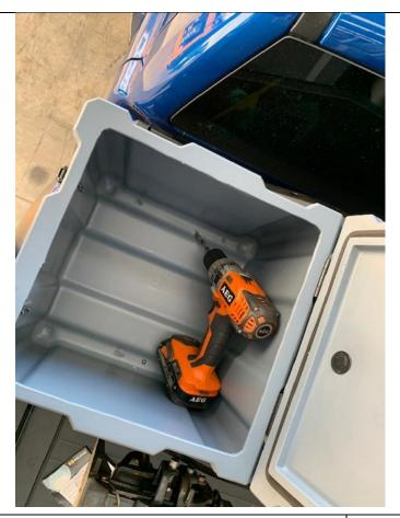
29. If fitting small space case to flat basket, you'll need to drill holes in from inside box and secure down. This will allow you to open the box without removing it, and prevent it from being stolen
