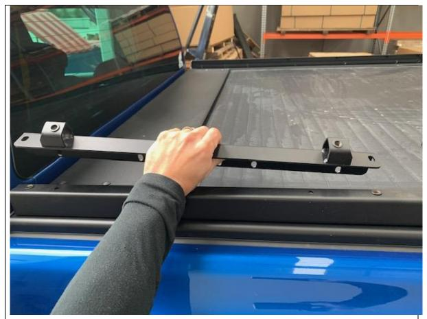
23. Drop Tub Rail assy on top roller shutter mount and secure with at least 4 M8 screws per side
