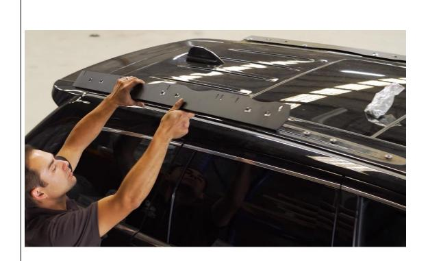
5. Lift steel rail onto roof ash shown. Repeat for other side
