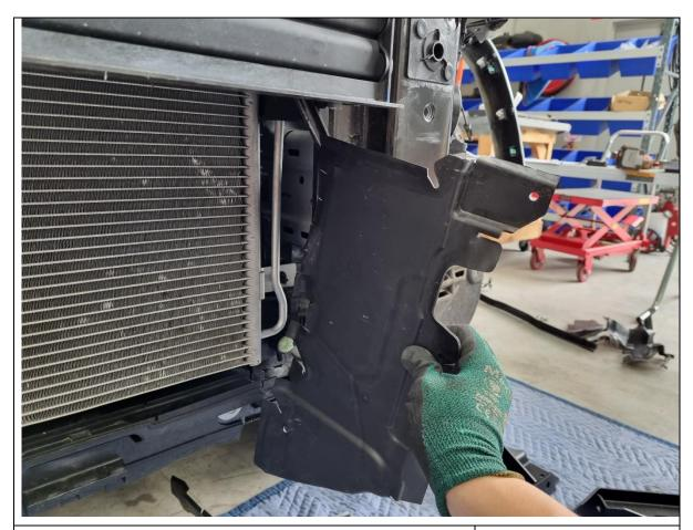
23. Unclip and remove the lower air dams with a flat head screwdriver or trim tool.
