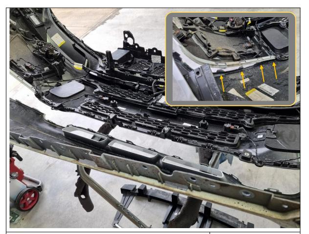
57. Unclip the lower half of the bumper from the main section.
