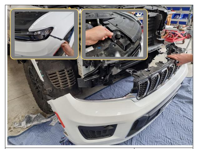
16. Remove the bumper by releasing the clips on either side and lifting the top flap of the grille over the bonnet rubber stops.
