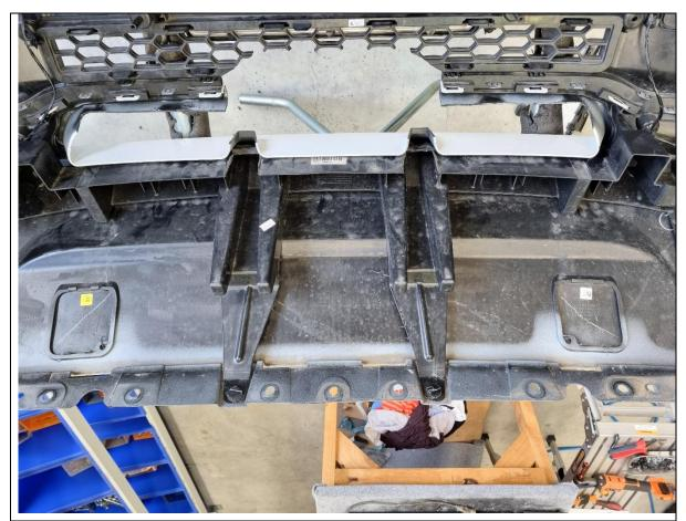
73. Reassamble the main bumper section, lower half and plastic inner support back together using the original fasteners.
