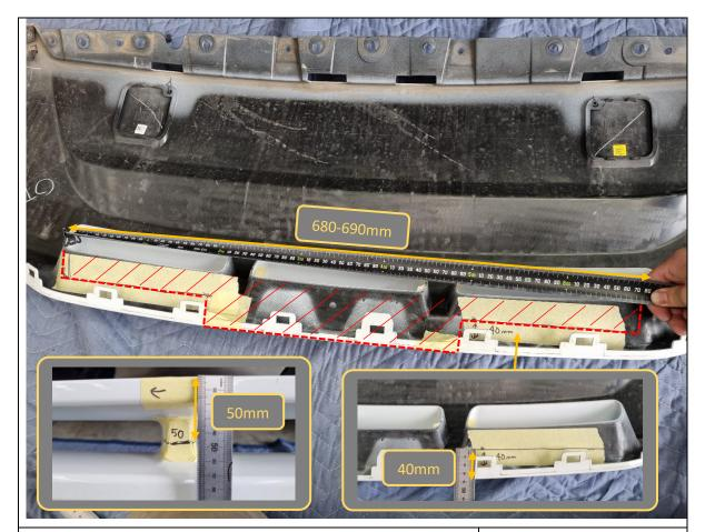
In top view, the overall width of the cutout must be 680mm+ to clear the cradle.
