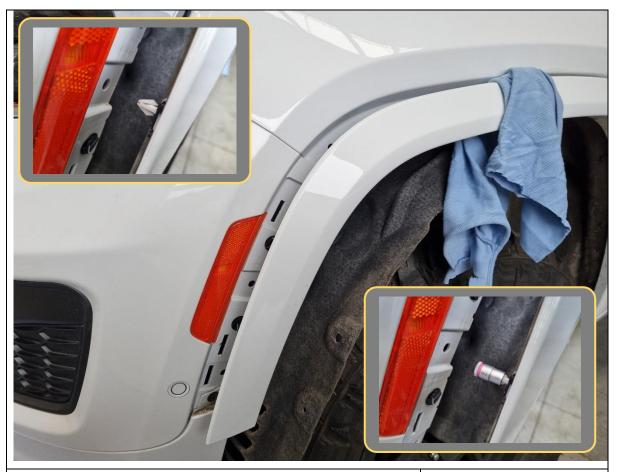
11. Pull and release the clips retaining the flare to the bumper + quarter panel.
