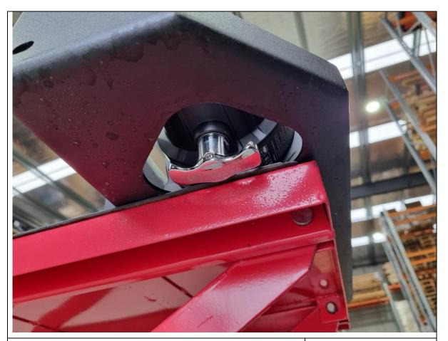
36. (OPTIONAL) When fitted with the Offroad Animal Pre Runner steel front bumper, the winch clutch lever can be accessed from below.
