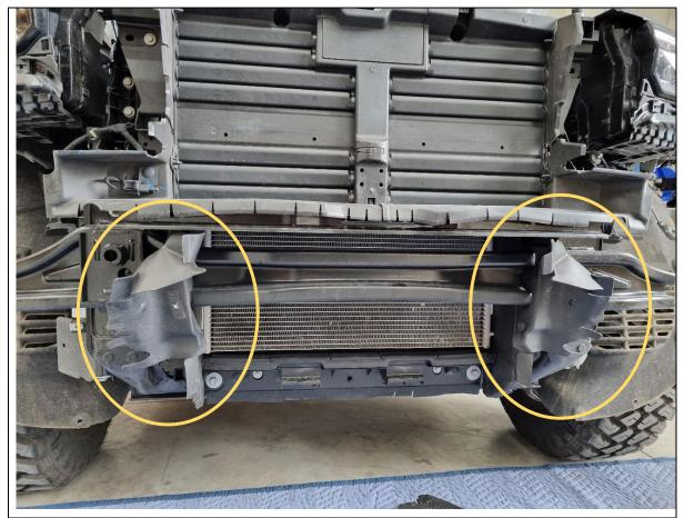
17. Unclip and remove the air dams with a flat head screwdriver or trim tool.
