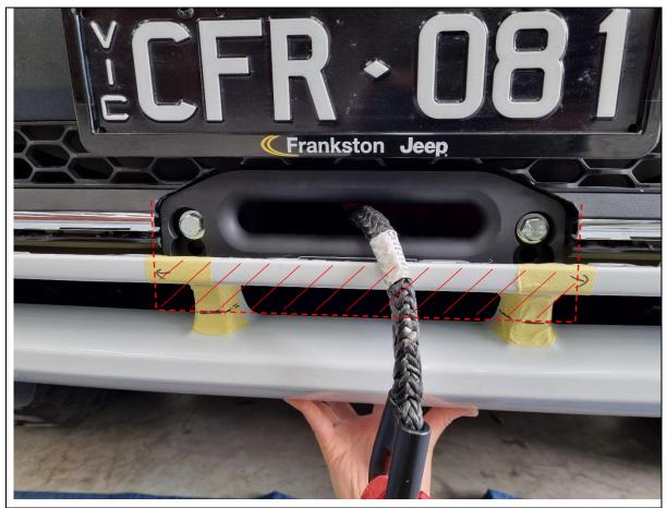
69. Hold the lower half bumper section to the vehicle and mark out where material needs to be removed for the hawse fairlead and cradle.
