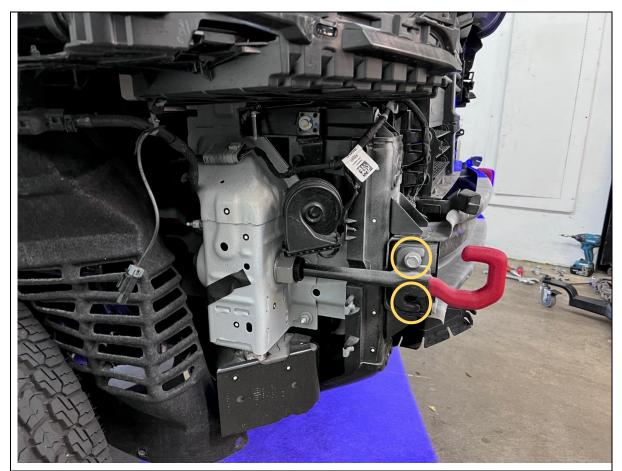
18. If factory tow hooks are equipped, remove the 2x 16mm hex head bolts on each side.
