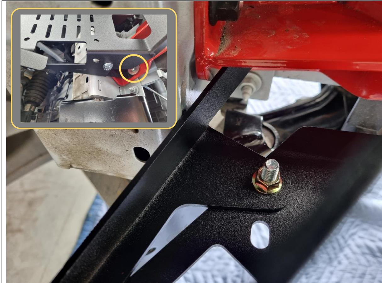
44. Fit the control box relocation support brace to the bottom flange of the relocation bracket and to the hole with the M8 lollipop nutplate used in Step 24 (see circled inset photo, recovery point is fitted in this example).
