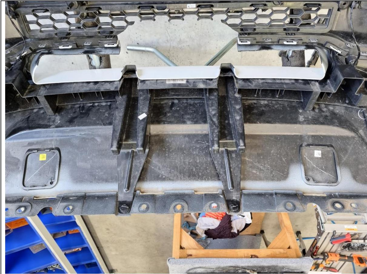
73. Reassemble the main bumper section, lower half and plastic inner support (Overland models only) back together using the original fasteners.
