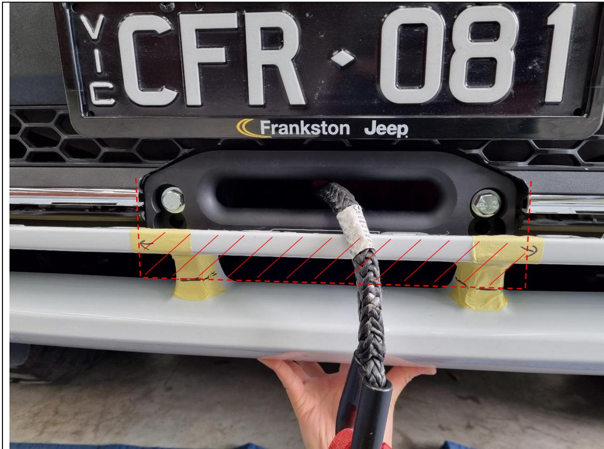
69. Hold the lower half bumper section to the vehicle and mark out where material needs to be removed for the hawse fairlead and cradle.
