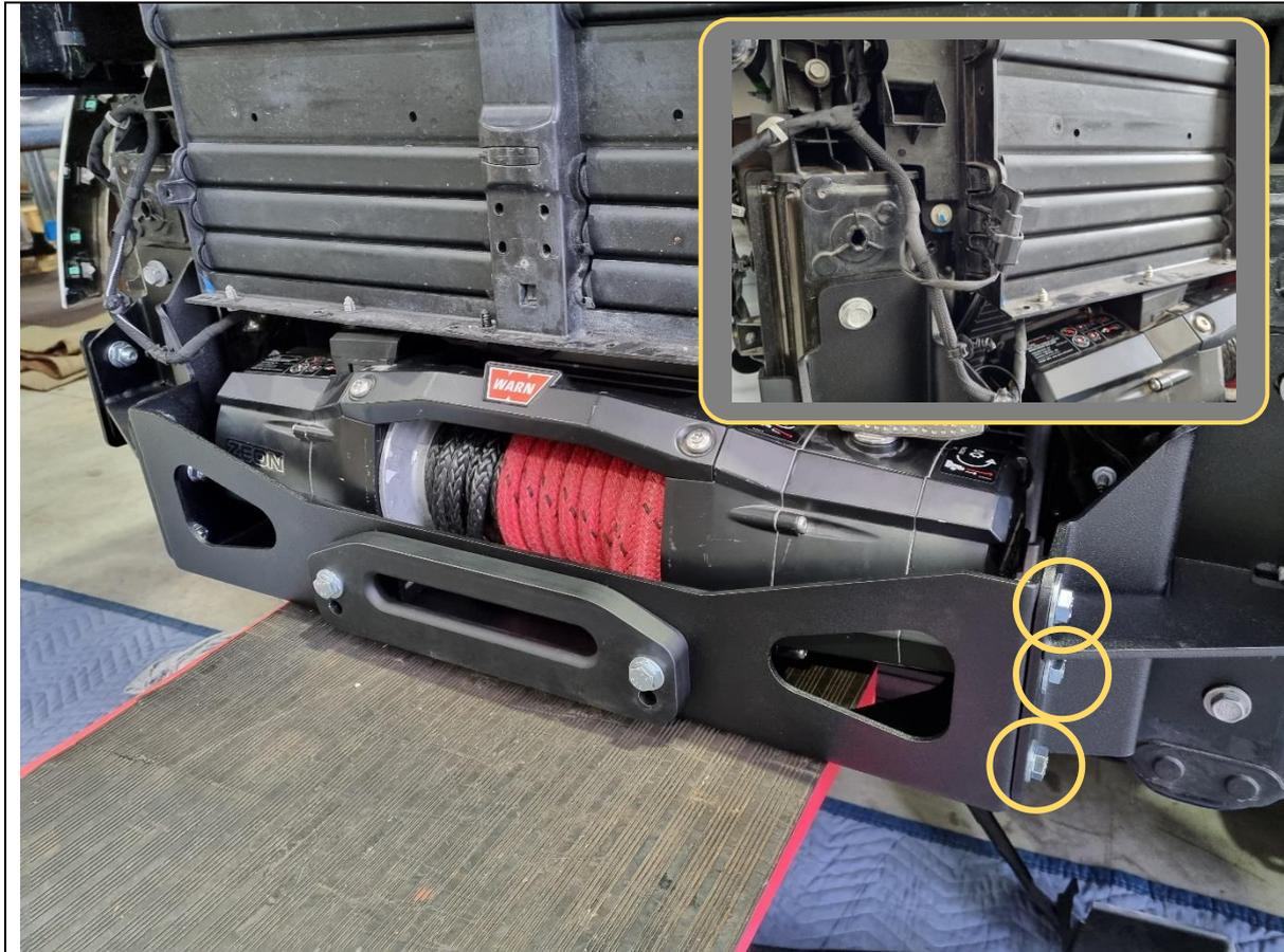
37. Fit the winch and cradle to the winch mount brackets using 6x M10x30 hex head bolts, flat washers and flange nuts.
