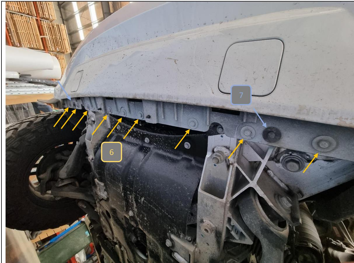
6. Remove 9x 10mm hex head bolts from the bottom of the bumper.
