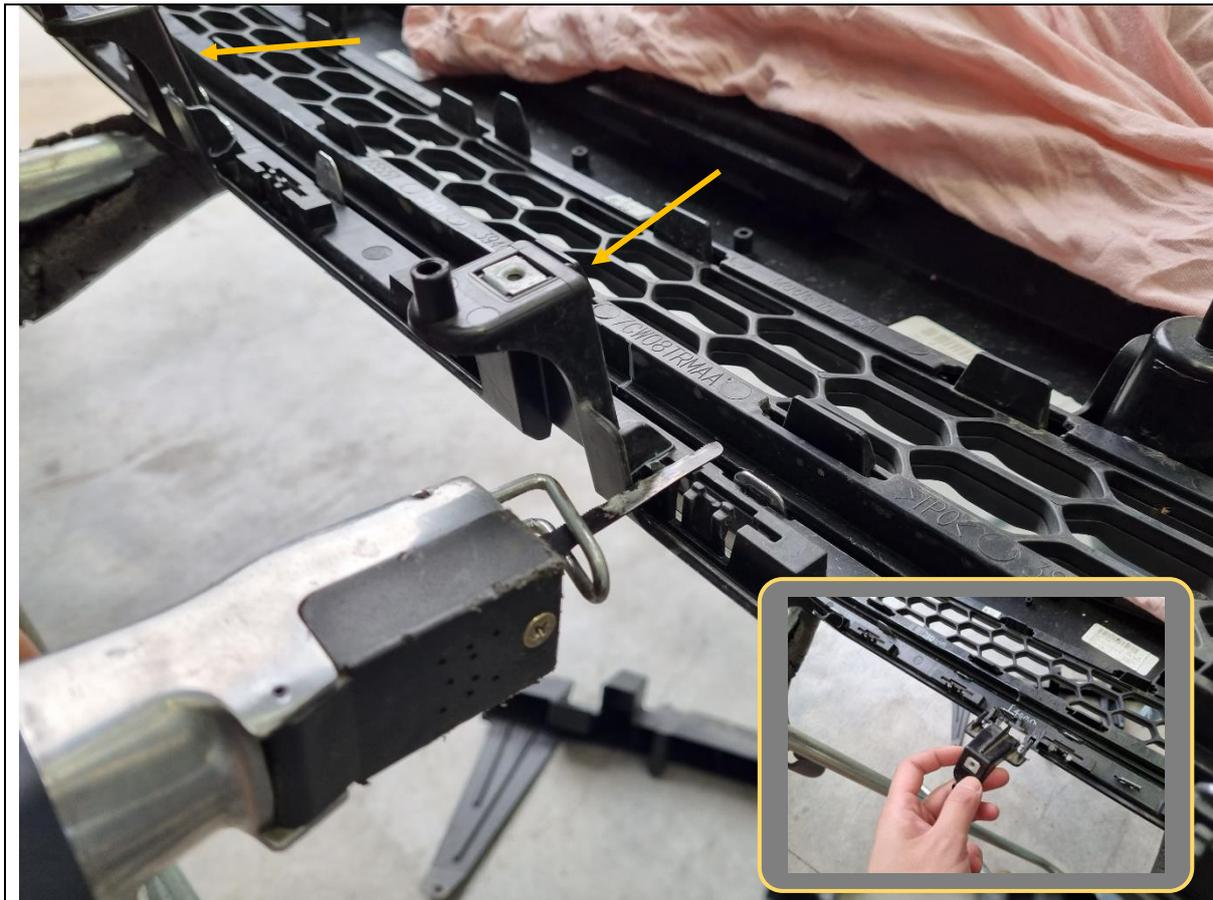
62. Protect any radars/sensors with a rag before trimming.
