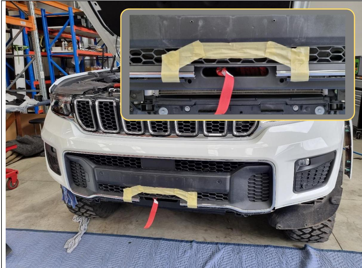
66. Fit the bumper back onto the vehicle.
