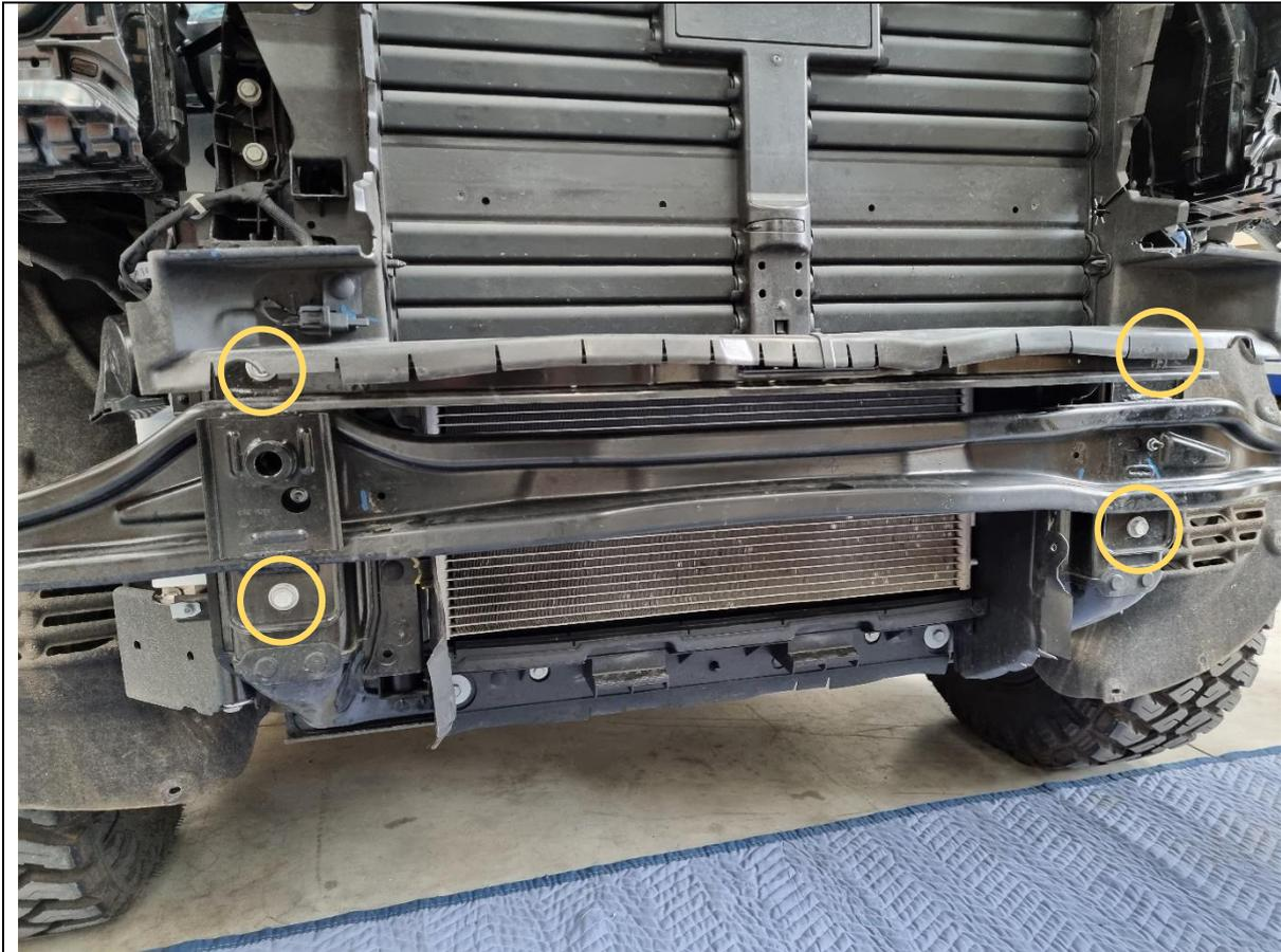
19. Using a 16mm socket or spanner, remove the 4x hex head bolts securing the impact beam to the body.
