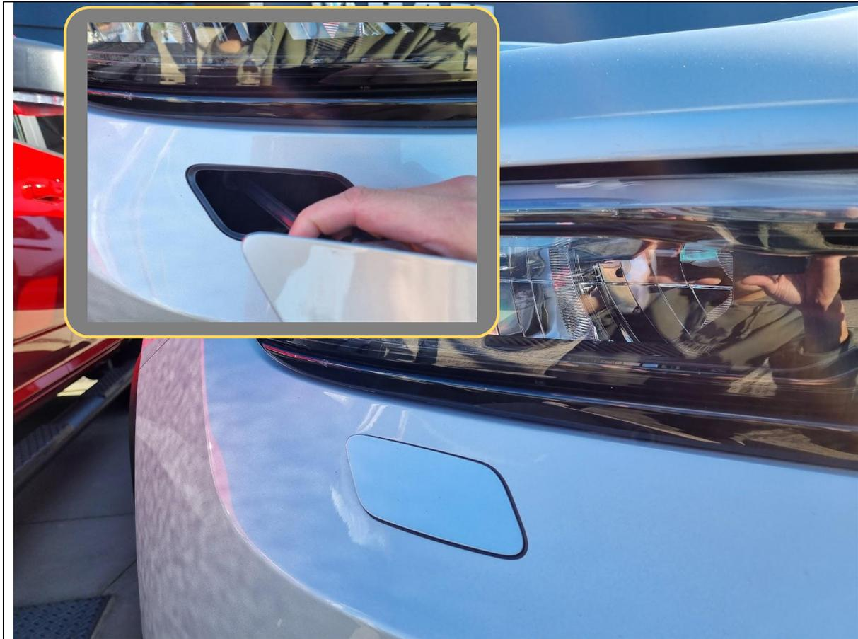
15. If headlight washers are equipped, pull out the plastic cover cap and unclip it from the plastic washer stem.
