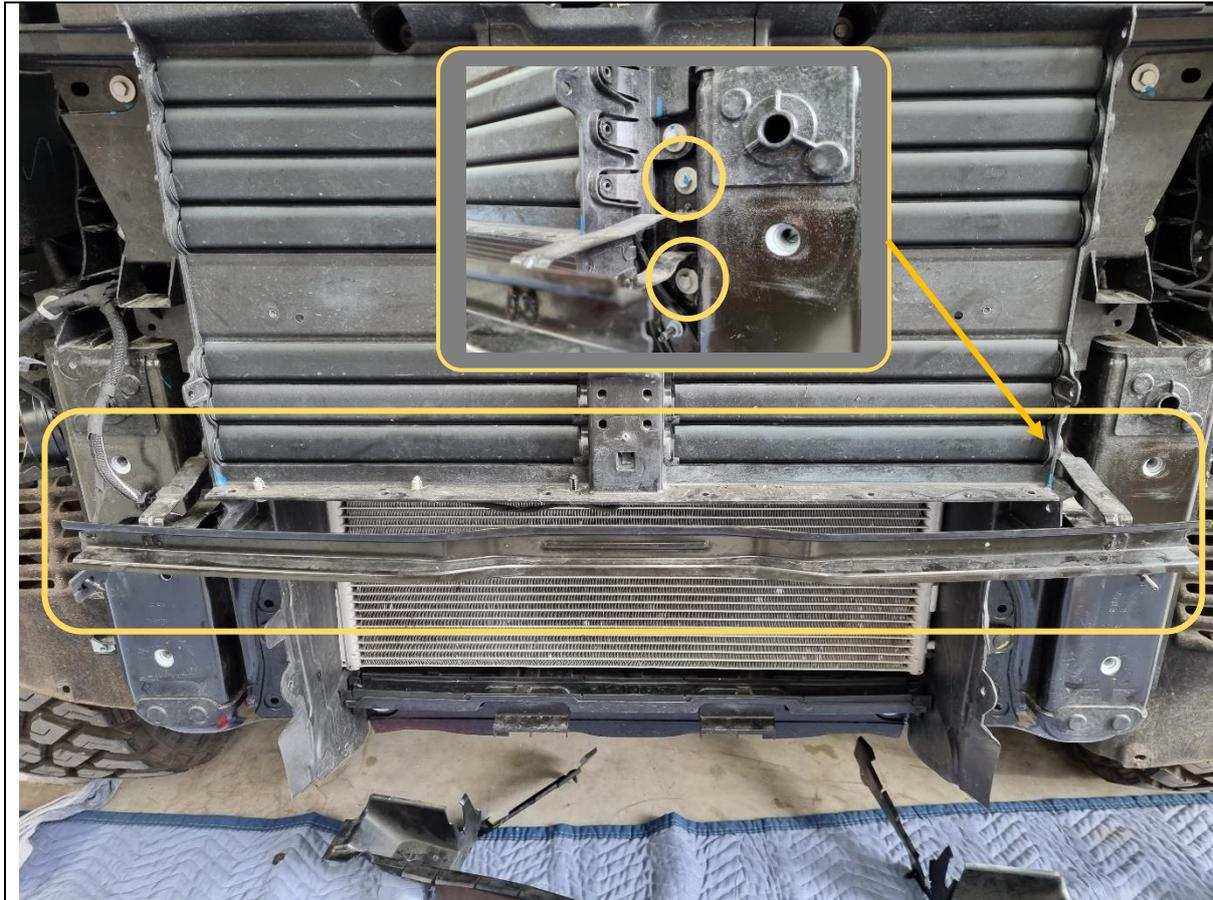
22. Remove the steel cross beam by removing the 4x 10mm hex head bolts securing it to the body (see inset).
