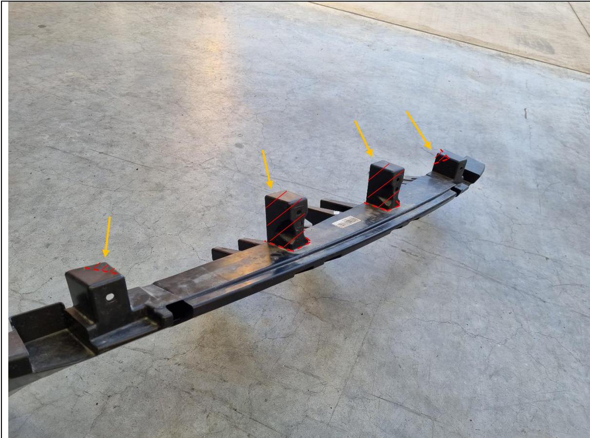
71. **Overland models only.** Cut off the middle two vertical posts on the plastic inner support.
