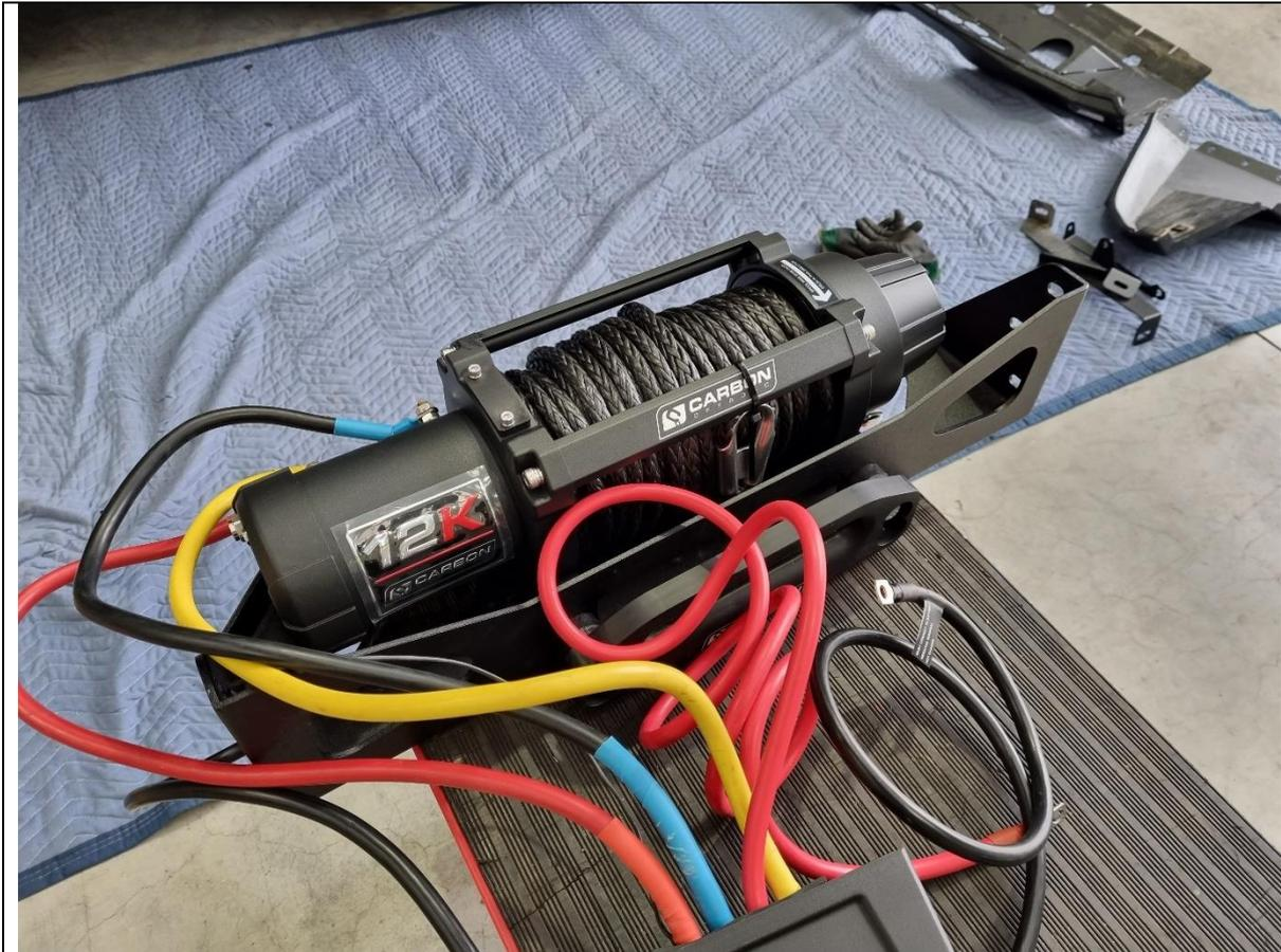
32. Fit the winch to the winch cradle using fasteners supplied by the winch.
