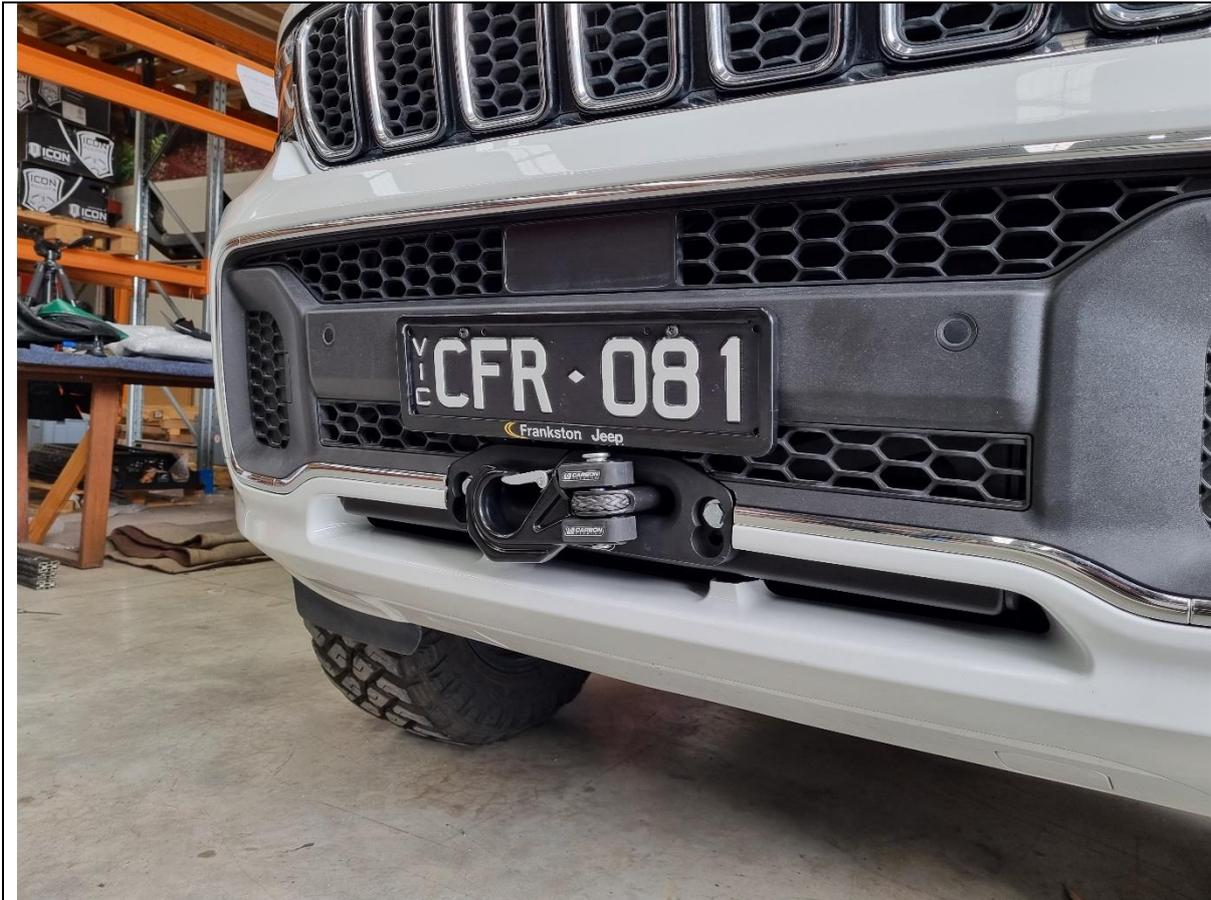
74. Refit the fully trimmed bumper back onto the vehicle. Reconnect all looms and washer hose lines. Then refit flares, inner wheel guards and radiator covers in reverse order to disassembly.
