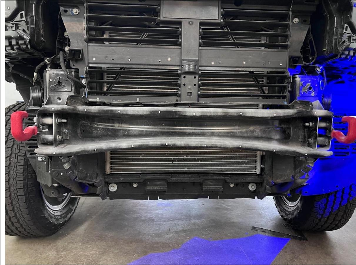
18. For vehicles with the same impact beam shape as the image above (i.e. vehicles equipped with factory tow hooks) and are not fitting an Offroad Animal Hidden Winch Mount, skip to Step 25.
