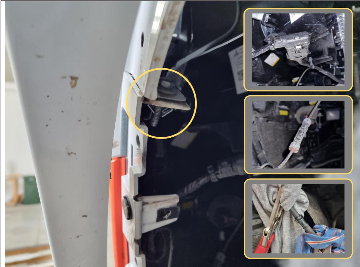
13. On both sides, remove the 10mm hex head bolt securing the bumper to the quarter panel.
