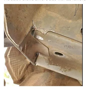
Note: Cuts made to the tub and the bumper bar must be sprayed with automotive touch up paint to prevent rust from exposed metal surfaces
