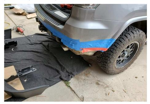
Remove the rear exhaust hangers (both exhaust pipes). Disconnect driver's side rear tail pipe (2 bolts) and let hang on outside hanger to make room for installing the bar and for accessing bolts near exhaust. The ride side exhaust can be pushed to the outside to gain access to the bolt. Lift the bar at an angle (down driver's side, up passenger side). Bring the passenger side up near mounting position. Lift over the hitch if equipped, and lift the driver's side into position
